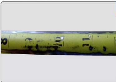
Bare metal showing on the blade; excessive wear on case exterior indicates the tape measure is worn out.
