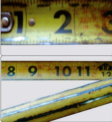
Rust and corrosion on blade or end hook indicates that the tape measure has been exposed to moisture or extreme conditions for long periods
