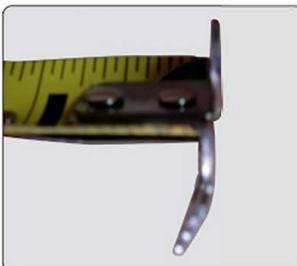
End hook is bent from tape being dropped, stepped on, or accidentally hit by another tool.
