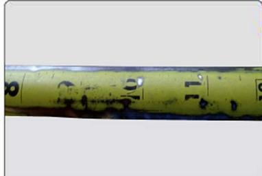
Bare metal showing on the blade; excessive wear on case exterior indicates the tape measure is worn out.
