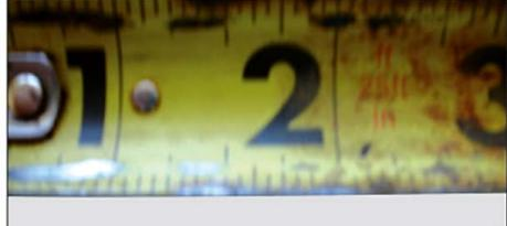
Rust and corrosion on blade or end hook indicates that the tape measure has been exposed to moisture or extreme conditions for long periods
