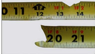
Blade torn by retracting at a high speed, broken by being stepped on or accidentally cut by a power/or hand tool.
