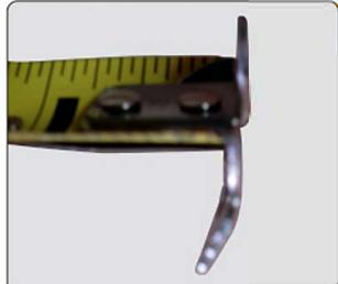
End hook is bent from tape being dropped, stepped on, or accidentally hit by another tool.
